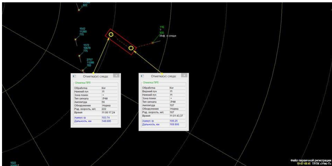
Figure 18 – Airborne object No. 116 in "an opposite direction" trajectory. The airborne object in the reference segment of the trajectory was observed steadily
