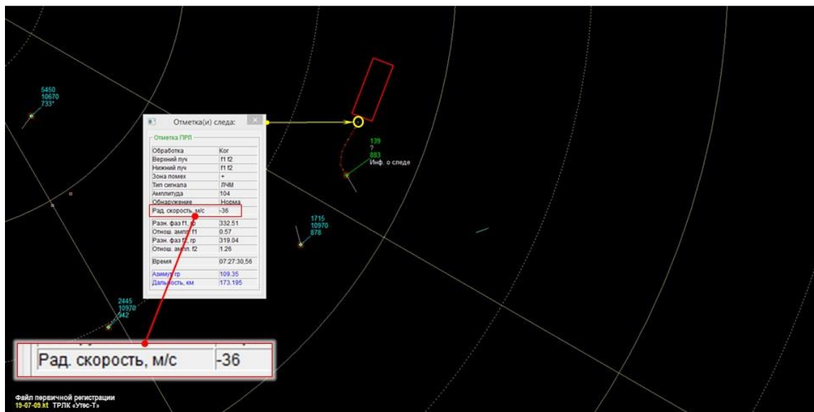
Figure 21 – Tracking of the reference airborne object after completion of the flight along a special trajectory simulating the missile flight from the southern direction
