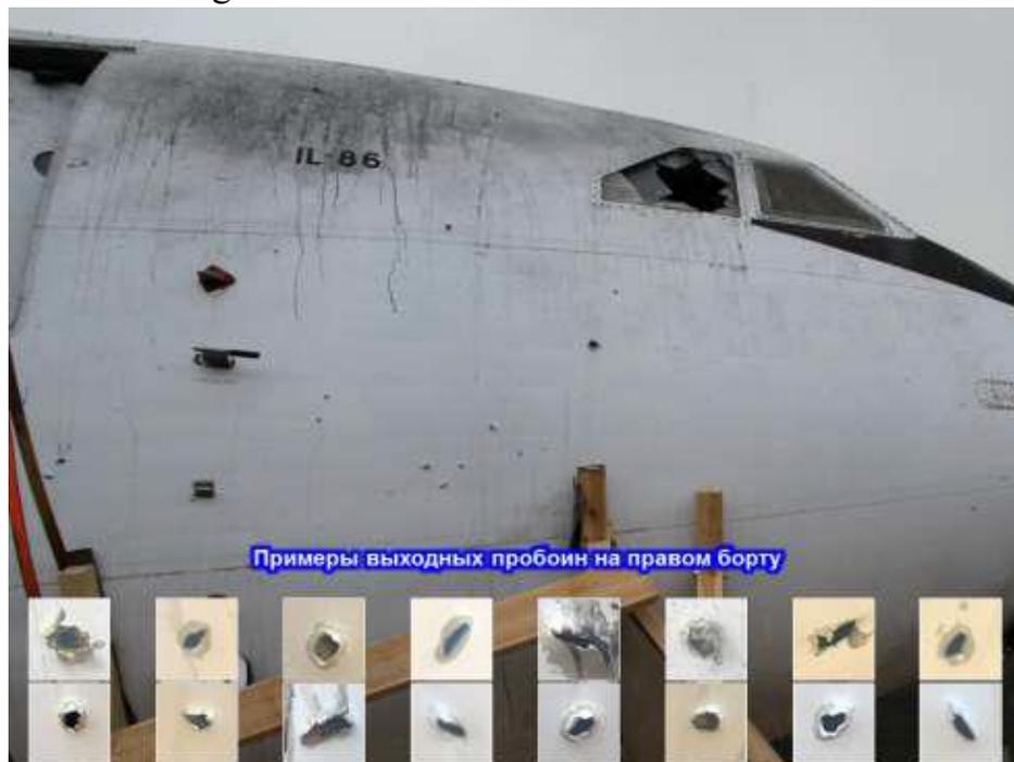
Figure 5.2.30 - Examples of through-hole exit punctures ("inside-out") on the starboard side of the IL-86 target aircraft
