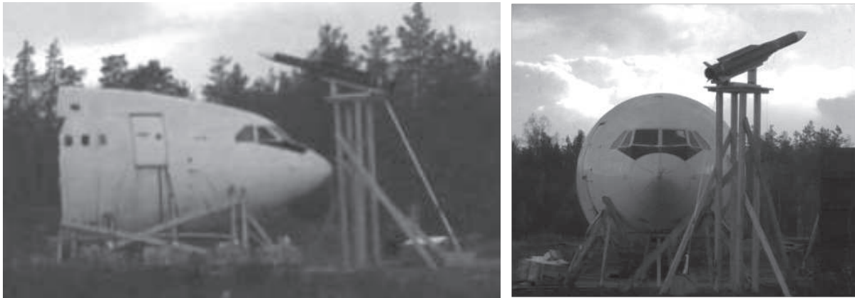
Figure 5. Target set-up of the second experiment, recreating the conditions indicated in the DSB report for the contact between the Boeing 777, flight MH17, and the missile
