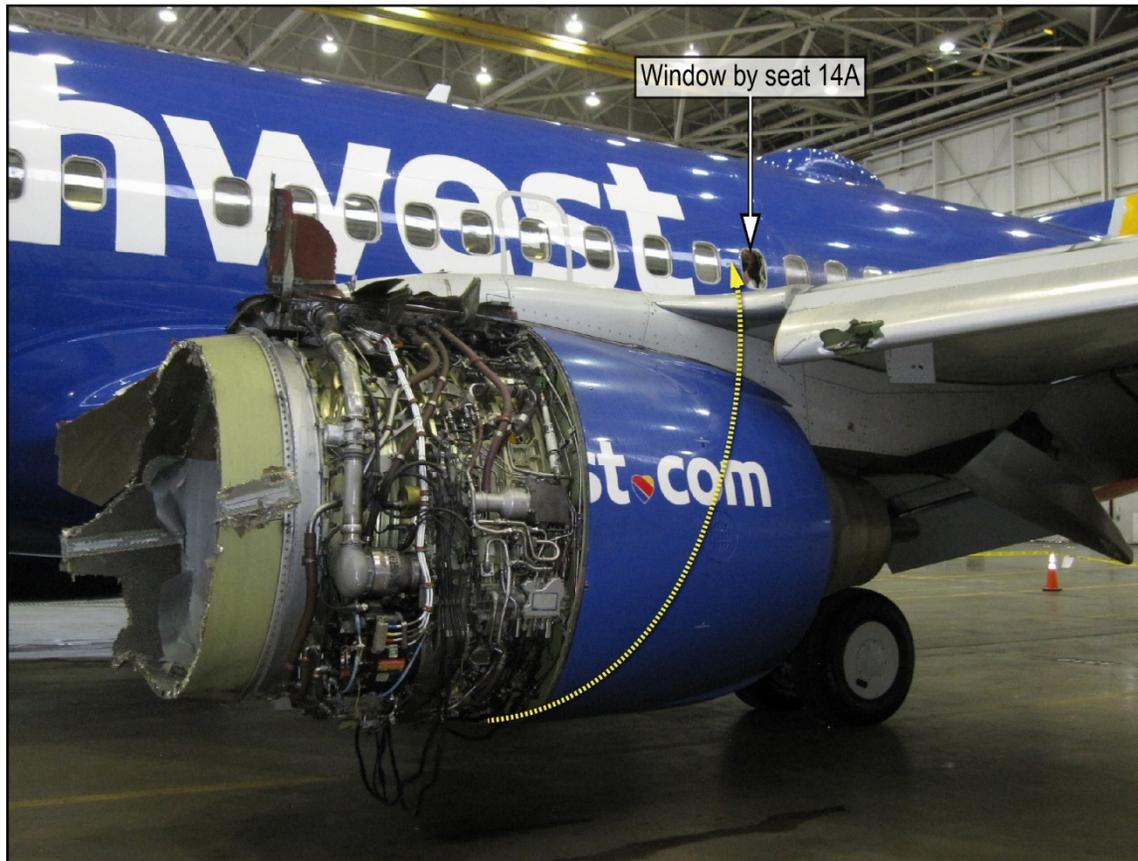
**Figure 22.** Trajectory of the inboard aft latch keeper during the accident sequence.
