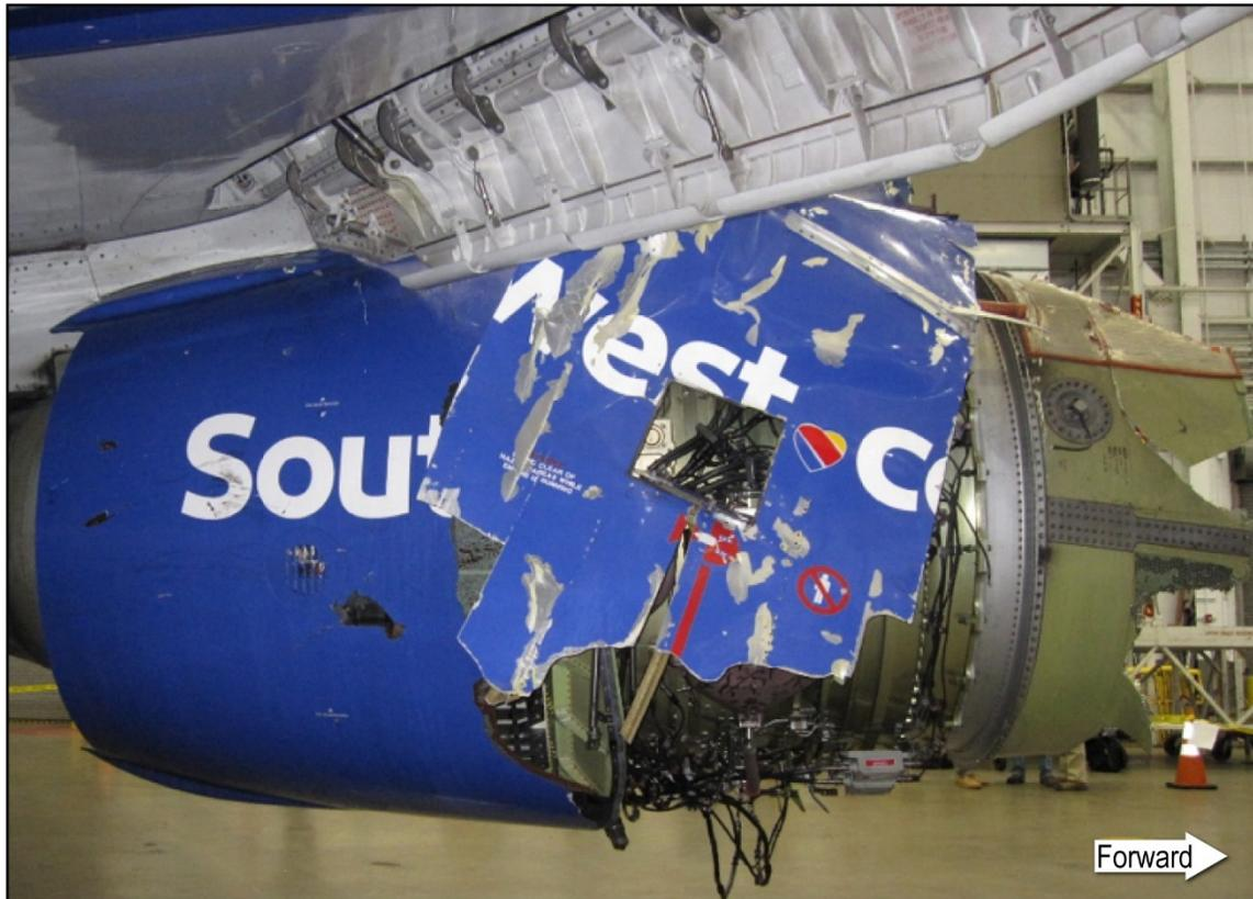
**Figure 9.** Inboard fan cowl damage.
