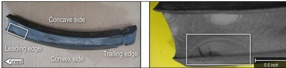
**Figure 7.** Fatigue indications on fan blade fracture surface.
