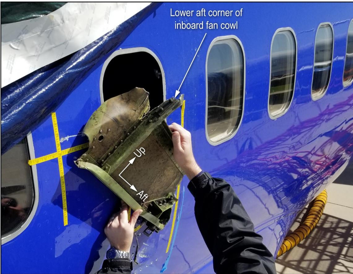
**Figure 6.** Lower aft corner of inboard fan cowl aligned with witness marks on fuselage.
