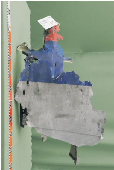
Figure 18: Part of fuselage left hand side showing holes and pitting. (Source: Dutch Safety Board)
