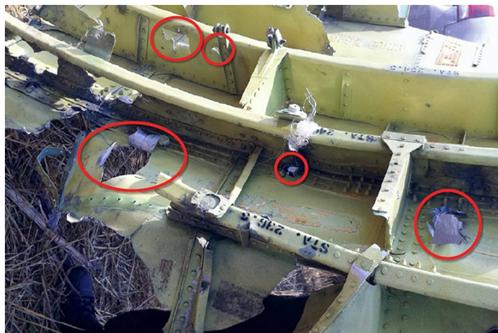
Figure 9: Part of the inside cockpit roof, indicating penetration with objects from outside.
