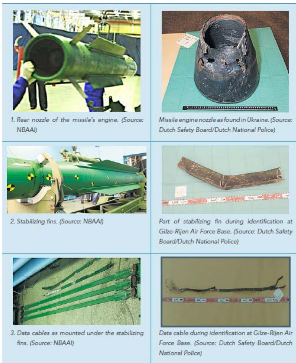
Figure 36: Weapon parts recovered. The parts are shown with sample photos showing their origin on a 9M38M1 surface-to-air missile.
