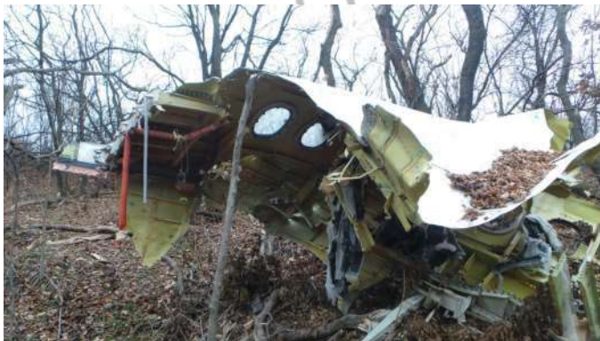
19 20 Figure 63 – Severely deformed fuselage structure aft of passenger door 3R, 21 including aft cargo door surrounding structure (source: DSB)
