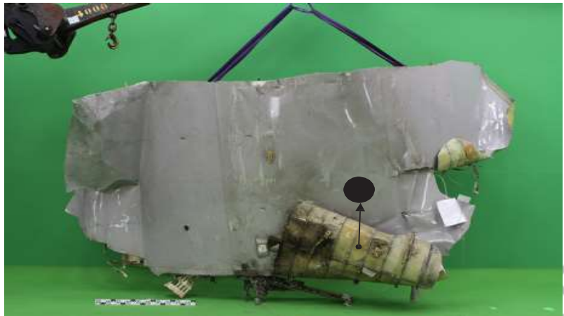
Figure 55 – Example of bending/peeling at a fracture line located along STA655 associated with the final separation between two pieces of wreckage.
