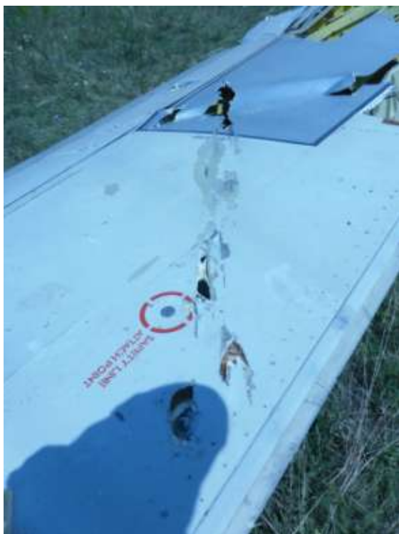
9 Figure 18 – Left wing tip with impact damage (Source: ATSB)
