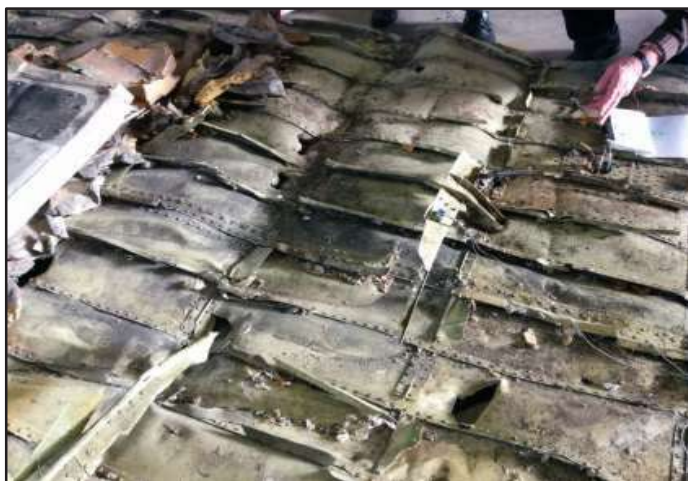
1 2 3 4 Figure 57 – Example of gross buckling of the lower fuselage skin panel near STA487.
