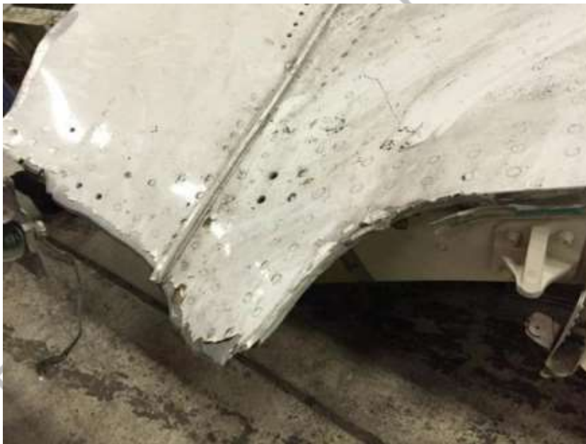
21 Figure 59 – Tensile overstress fracture at the upper right door corner of passenger 22 door 3L 23
