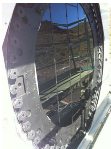
Figure 2.19: Filter for moonlight observations.
