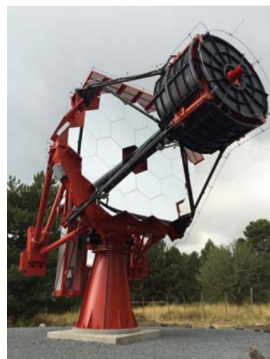
(e) Dual-mirror SST prototype on Mount Etna.
